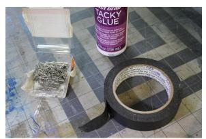
You may assemble your model using pins, tape or glue. Pins work best with foam core models, whereas tape can be used for any kind of material. The benefits of using either tape or pins (or a combination of both) is that it is easy to disassemble the model afterwards. This is convenient for both storage and shipping. Glue is cleaner but it makes the model permanent.
